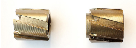
15mm cutter (left) and 16mm cutter (right; with inserted cutter spacer). Note, the cutters come pre-installed in the Drill Jig.
