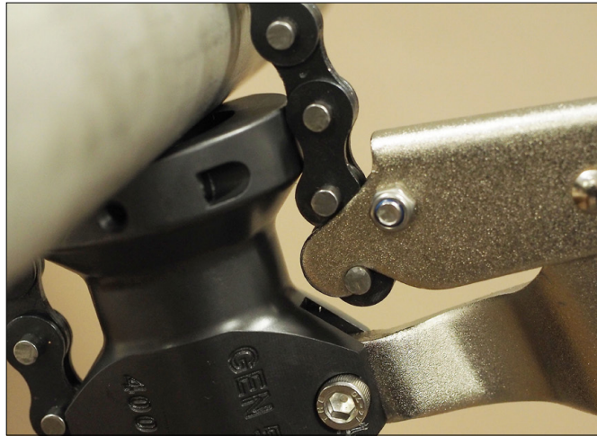
Above: The clamping chain is secure, in a central position, and is not touching the engaged vice grip or the central section of the cutter assembly.
