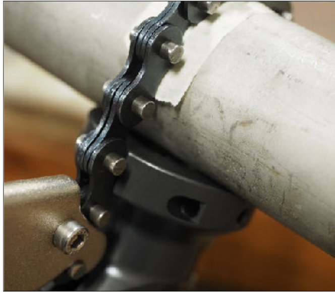
Fig. 6.2 - 6.5 Align clamp body with the tape and engage the chain hook and clamping chain. Ensure the level bubble remains centered.
