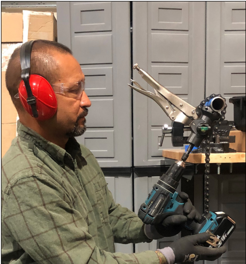
Above: The THETA 750 SNAP Drill Jig in use. Proper use of the Drill Jig will result in a significantly faster and more professional finish.
