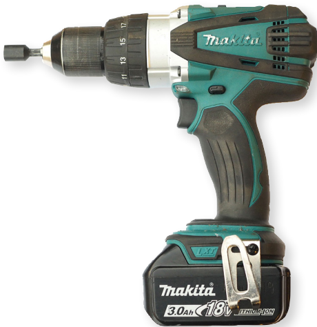
A battery-operated (cordless) drill; 400RPM maximum. We recommend using a large battery pack and spares.
