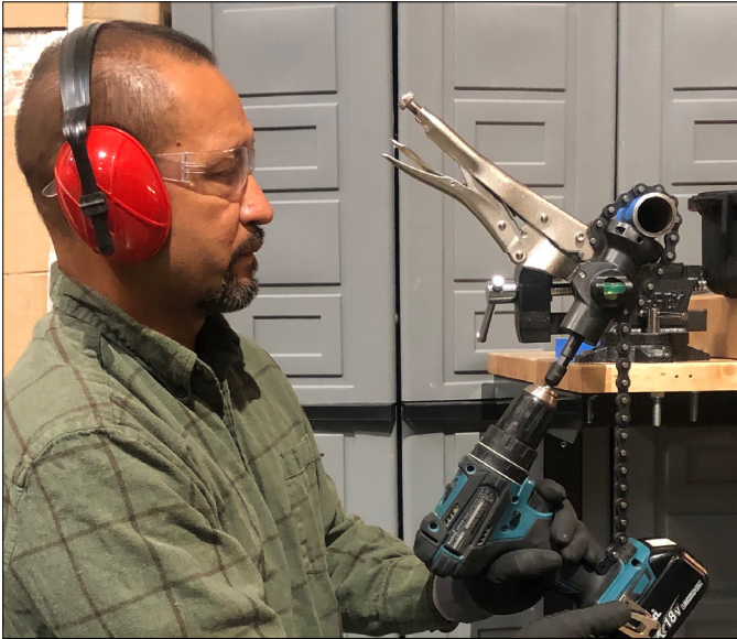
Fig 8.1 Do NOT force/push the drill. Use light pressure only to keep the socket engaged.
