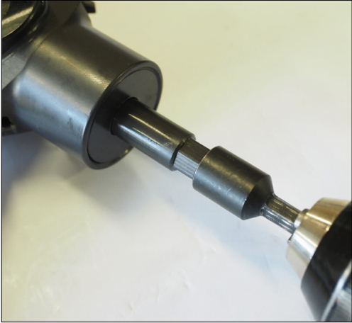
Fig. 2.1 If cutters are pre-installed, use your drill to ensure that both the hex drive and cutter end of the cutter assembly are fully retracted.
