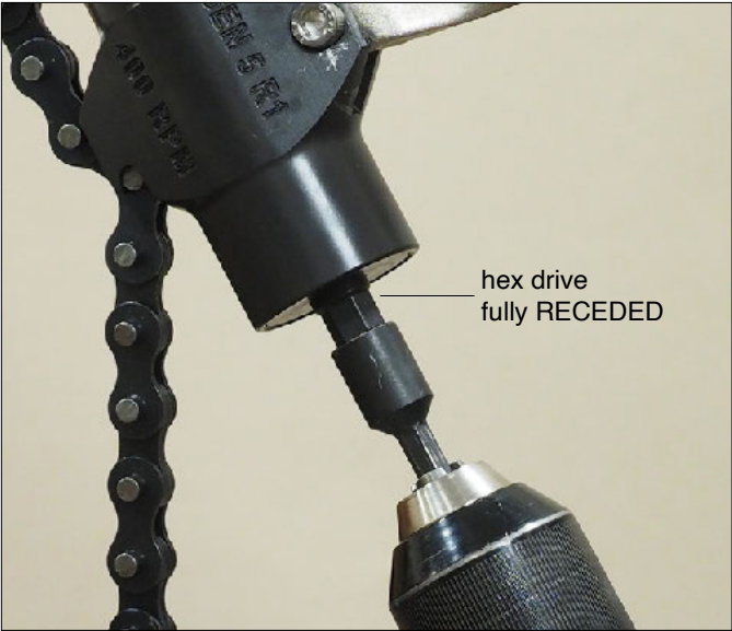
Fig 8.2 STOP drilling once the hex drive has fully receded inside the Drill Jig.
