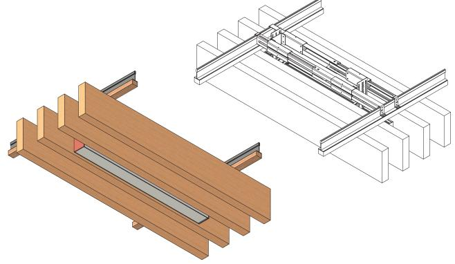
LONGER RUNS ZETA-PLS FIXTURE SETUP WITH 48" MOUNTING BAR SET (SHOWN 8 FOOT FIXTURE EXAMPLE) APPEARANCE BELOW CEILING
