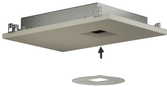
1. Fasten mud frame to ceiling.
