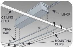
1. Can be used with any of the Emergency Battery Backups. Must be ordered as a separate line item.
