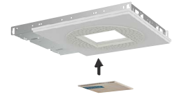
2. Insert protective cover (included). Apply joint compound over the mud frame.
