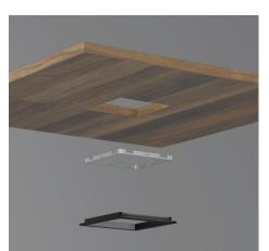
1. Insert Millwork Mounting Bracket using the included Plastic Spacer for proper depth positioning.
