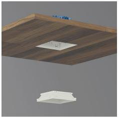
5. Insert Bezel to finish the installation.
