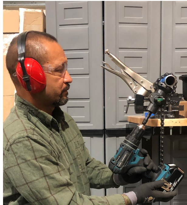
Fig 8.1 Do NOT force/push the drill. Use light pressure only to keep the socket engaged.
