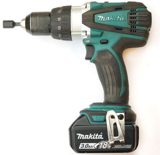
A battery-operated (cordless) drill; 400RPM maximum. We recommend using a large battery pack and spares.
