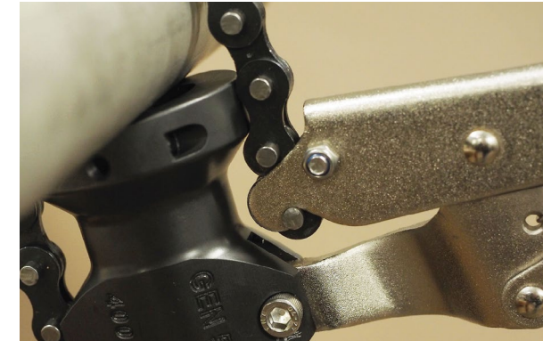
Above: The clamping chain is secure, in a central position, and is not touching the engaged vice grip or the central section of the cutter assembly.
