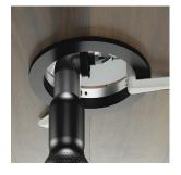
2. Use the included C-Clamps to temporarily hold the Plastic Spacer in position. Fasten the included wood screws into the Mounting Bracket using a right-angle impact driver (supplied by others)
