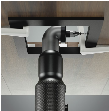
2. Use the included C-Clamps to temporarily hold the Plastic Spacer in position. Fasten the included wood screws into the Mounting Bracket using a right-angle impact driver (supplied by others).
