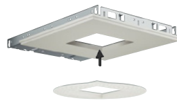
1. Fasten mud frame to ceiling.
