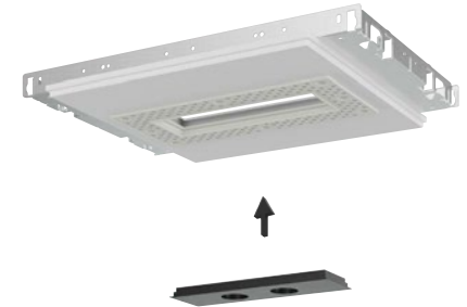
2. Insert protective cover (included). Apply joint compound over the mud frame. Finish, paint, and remove insert.
