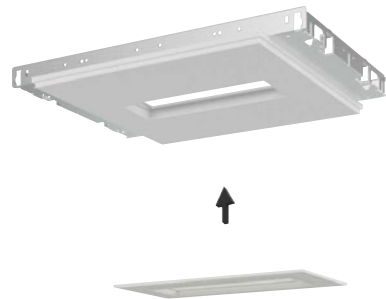
1. Fasten mud ring to ceiling.
